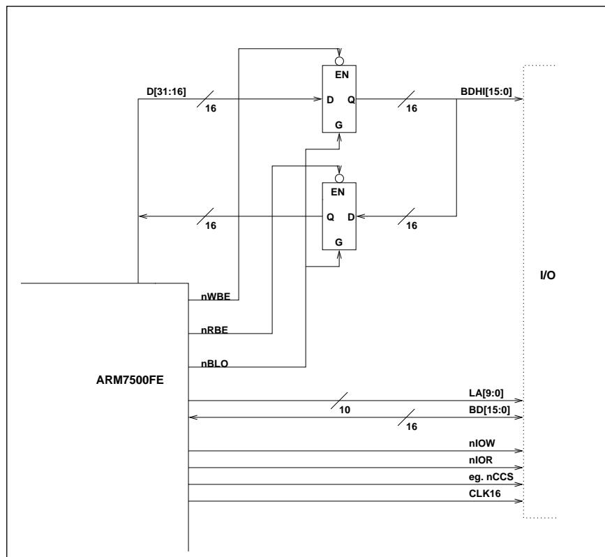
*Figure D-1: 32-bit I/O interface*
