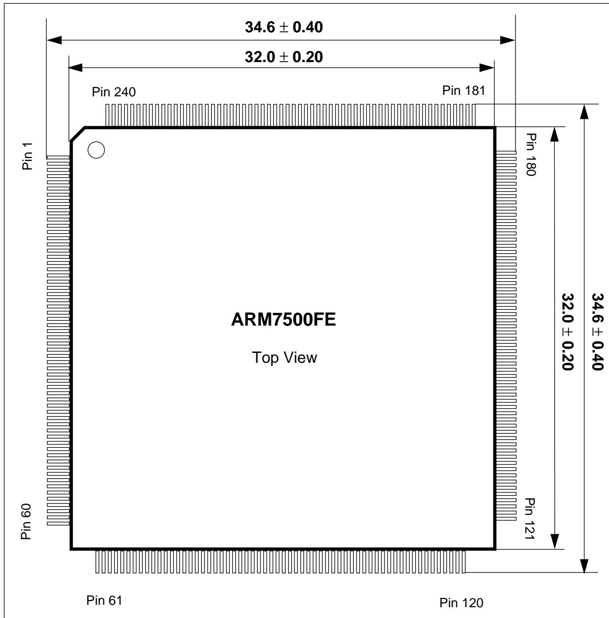
Figure 23-1: Pin diagram for the ARM7500FE
